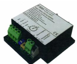
TSRL is an electronic relay for switching transformers. Using its patented soft start-up operation it activates one or more single – phase transformers open-circuited or on-load without inrush. By the use of the soft start-up operation the inrush is not only bordered but avoided.
