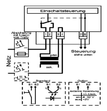
The TSRL biases the transformer for a short time before every switching-
